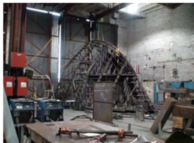
**Inverted Hull ribbing is welded into shape**
